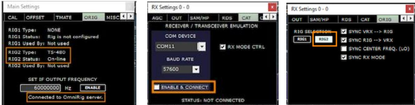
In RX SETTINGS, CAT tab, make sure “Enable & Connect” is **NOT** checked. On the ORIG tab select RIG2.
